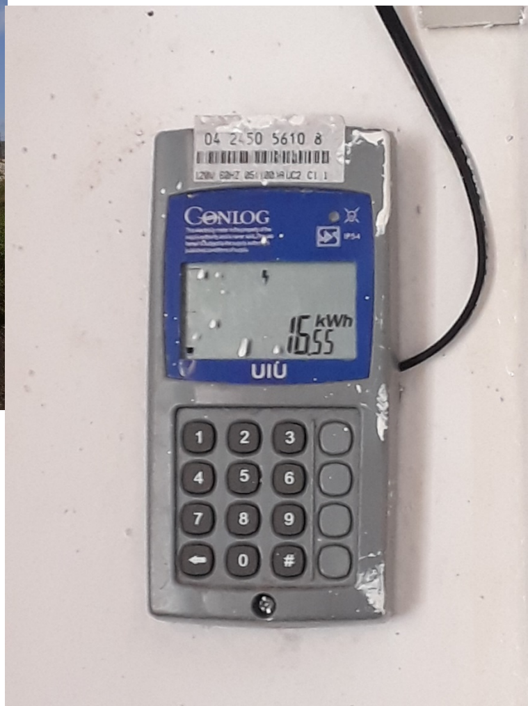
Image of a reading frame of a prepaid Coteaux meter indicating in real time to the user the number of Kwh remaining on his account. (Case of the CEAC Micro-network, South Haiti)
